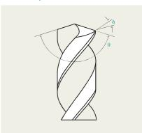
Rake angle: Cutting angle ( $\theta$ ): 120-140 deg Clearance angle ( $\delta$ ): 10-20 deg Feed speed: 60-300mm/min
